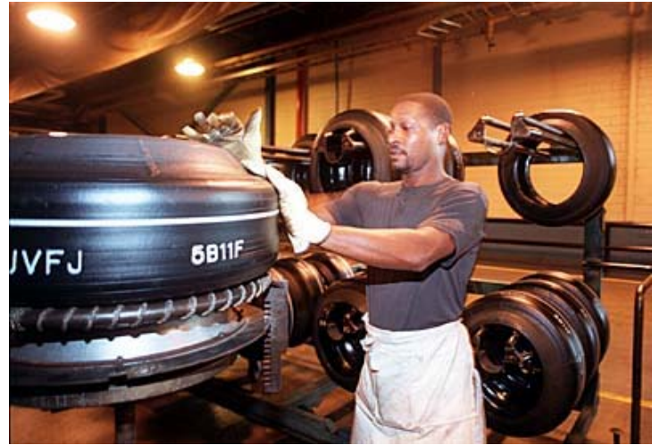
Firestone/Bridgestone truck tire prior to curing
